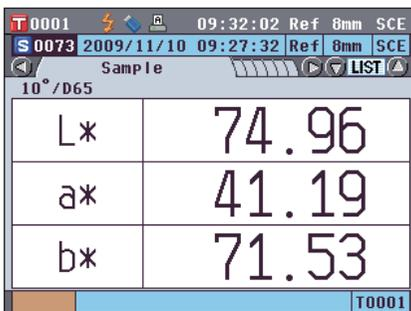
The screenshot shows the 'Sample Data Function' window with a table of sample data. The table has two columns: the first column contains labels (L\*, a\*, b\*) and the second column contains numerical values (74.96, 41.19, 71.53). The table is titled 'Sample' and '10°/D65'.
